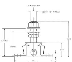
27166 Marine Mounts are compact, captive marine isolators designed to support light to medium loads from 138-750 lbs. per mount.
